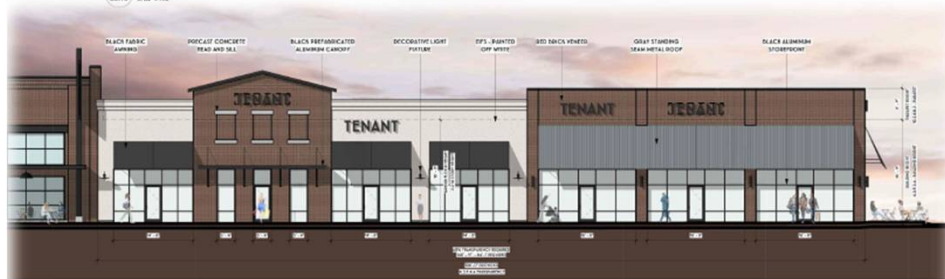
3 TYPICAL SHOPS - FRONT ELEVATION - WEST 44.11 1/2" = 1'-0"
